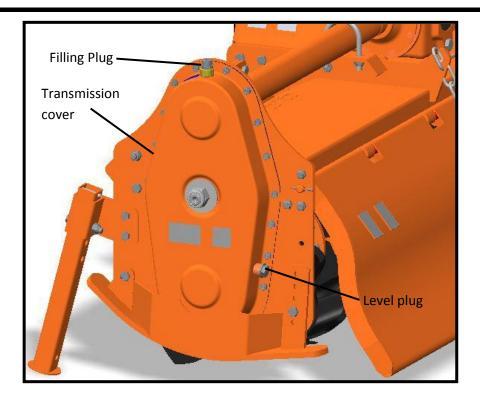
Check the oil level every 50 hours, making sure it reachs the level plug on the transmission cover. If the oil is below this level, fill up oil till restore the level.
