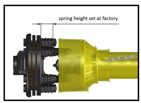
An adjustment can be done, however, when the clutch slipping is too frequent, which means that the calibration is too low.
